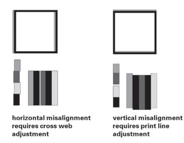
When the black box prints without any color shadows and the block pattern appears correctly aligned, the color alignment is optimal.
